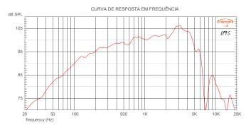
CURVA DE RESPOSTA NO EIXO FRONTAL A 1W/1M OBTIDA COM ALTOFALANTE EM CAIXA SELADA DE 390 LITROS EM BAFFLE INFINITO (HALF SPACE)
